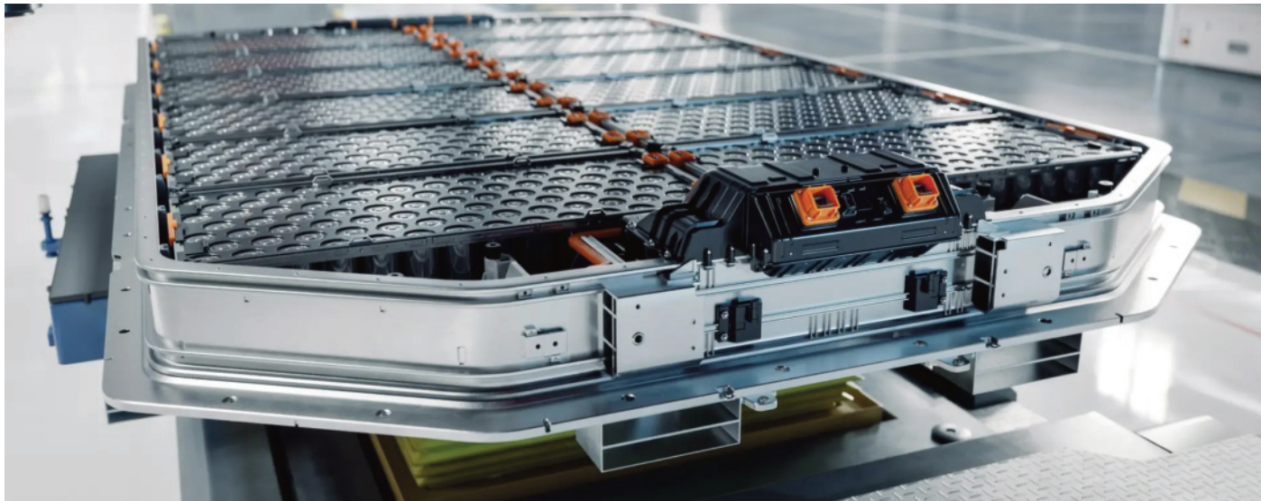
Fig. 1: Typical battery pack prior to assembly within a vehicle
