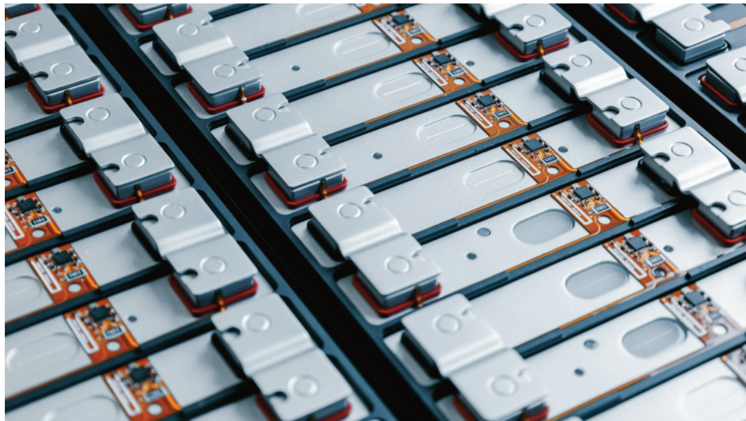
Fig. 2: Cell monitors fitted to EV cells
